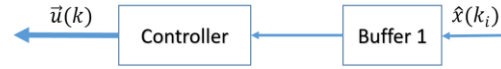
Fig. 2. The internal structure of the predictive controller For the system without time delay, the control signal is generated based on the equation
