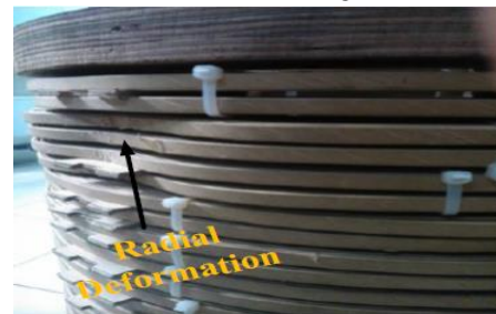
Fig. 2. Radial deformation on the transformer winding
