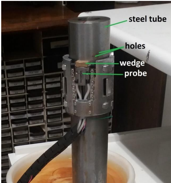
Fig. 8. The experimental setup, constructed by Niroo Research Institute (NRI) [34].
