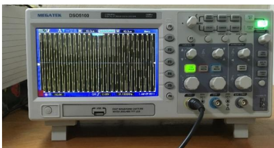
Fig. 14. An example of the output signal (two ends of the induction coil) produced in the oscilloscope.
