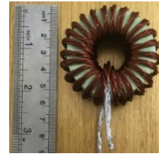
Fig. 8. The constructed inductor for L_1 and L_2 .
