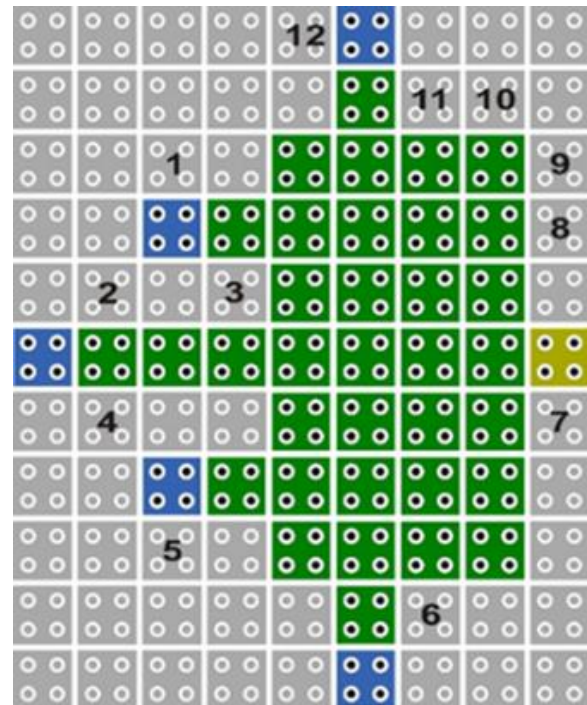
Fig. 11. The proposed five-input fault-tolerant majority gate circuit along with the analyzed points for redundancy fault.
