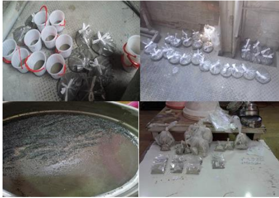
Fig. 4. Sampling and sieve analysis steps
