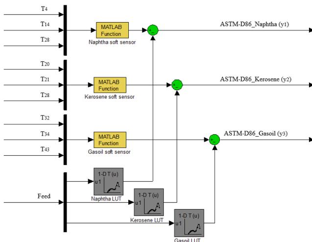
Fig. 6. Lookup table models in soft sensing structure
