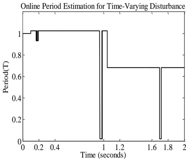
Fig. 8. Adaptive period estimation of two different periodic disturbances.
