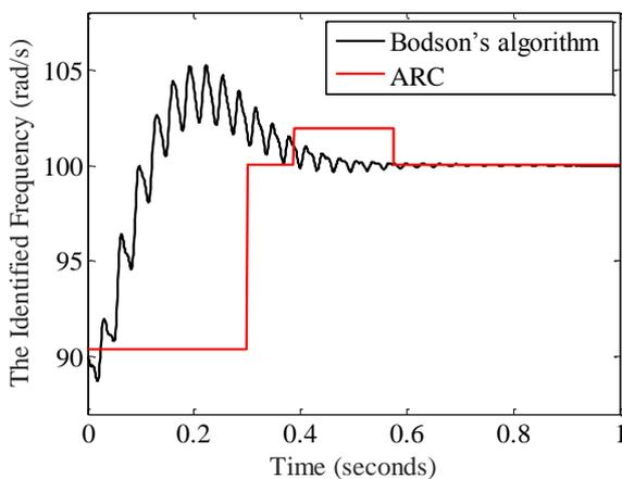
Fig. 10. The frequency estimation by Bodson's algorithm and the proposed approach
