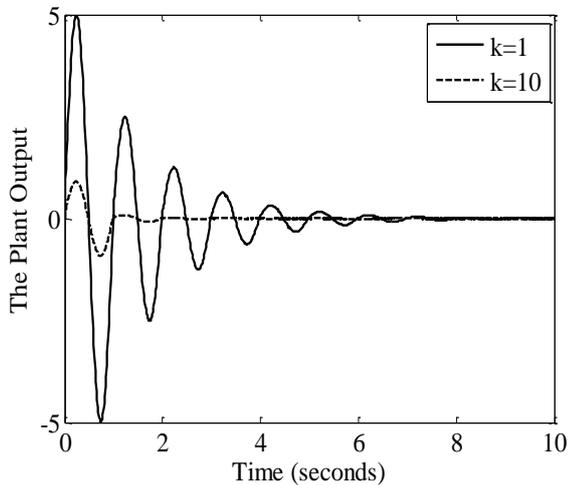
Fig. 4. Disturbance rejection for the previous case by new disturbance amplitude.
