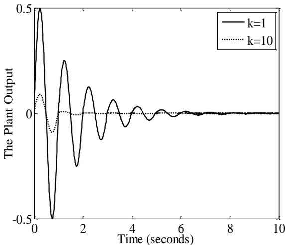
Fig.3. Disturbance rejection for different values of  $k$ .
