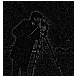
High Frequency Image (High Frequency Component)
