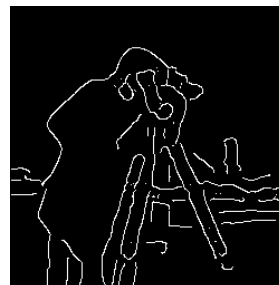
Extracted edges using canny method
