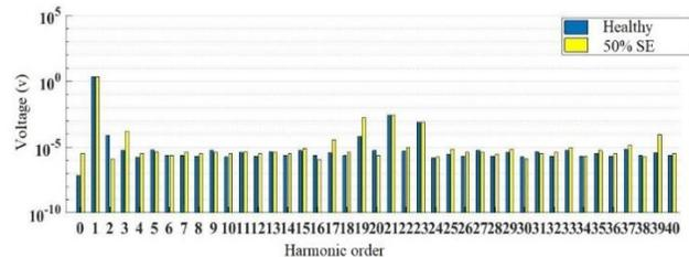
Fig. 7. Sine winding harmonic components under the healthy and static fault state
