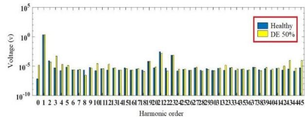
**Fig. 11.** The frequency spectrum of the voltage signal in the healthy state and under dynamic eccentricity states
