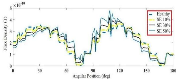
**Fig. 9.** Air gap flux density waveform under different static eccentricity values
