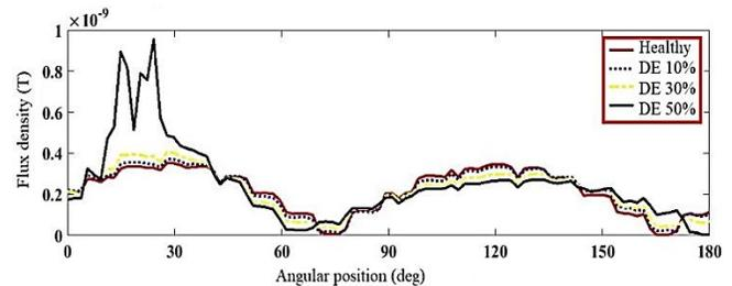
Fig. 13. The flux density of the air gap under dynamic eccentricity
