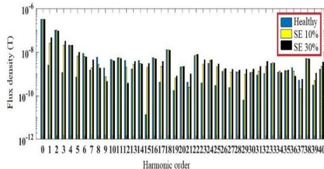
**Fig. 10.** The frequency spectrum of the air gap flux density signal in the healthy state and under static eccentricity states.
