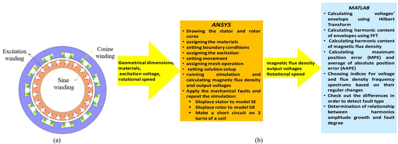
Fig. 1. (a) The schematic of the studied resolver (b) Schematic flowchart of the simulation procedure
