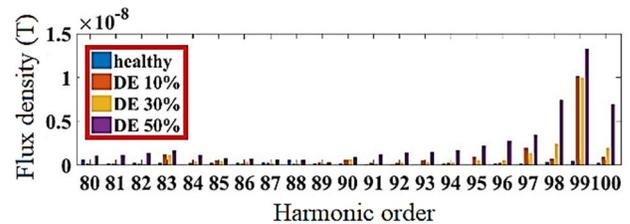
Fig. 14. Flux density amplitude frequency spectrum under dynamic eccentricity.
