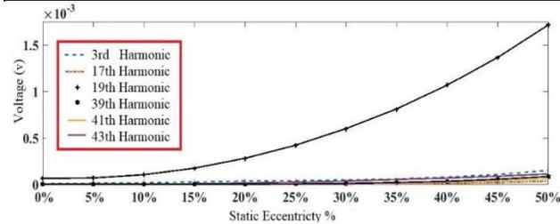
**Fig. 8.** Exponential increment in the amplitude of harmonics of flux density versus static eccentricity percentage
