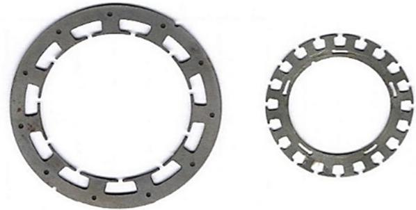
Fig. 3. Core sheets of studied resolver: (a) Stator sheet and (b) Rotor sheet
