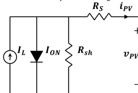
Fig. 2 The dynamic equivalent cell model.
