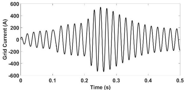
Fig. 13 Grid current in phase a,  $I_a$ , for the RHC during three-phase short-circuit fault.
