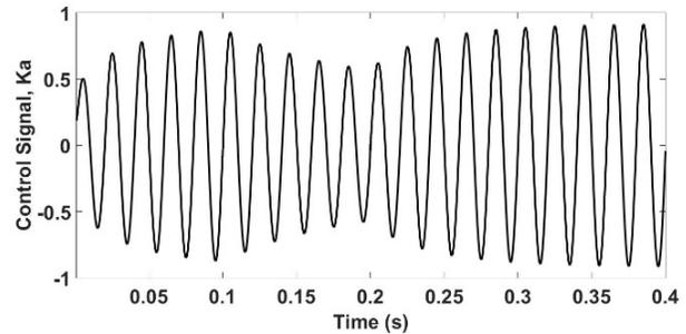
Fig. 10 Control signal in phase a, Ka, for the RHC by considering uncertainties (change in irradiation and ambient temperature).
