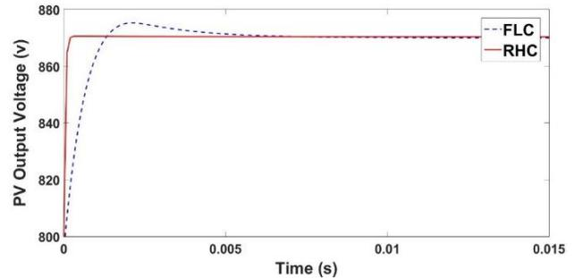
Fig. 4 Comparison of PV output voltage for the two controllers in standard atmospheric conditions.
