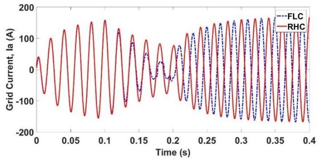
Fig. 11 Comparison of grid current of phase a for the two controllers by considering grid current (change in irradiation and ambient temperature).
