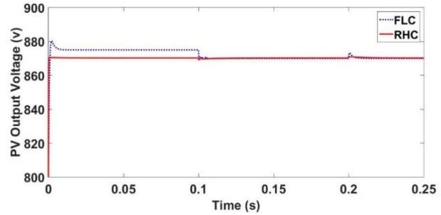
Fig. 9 Comparison of PV output voltage for the two controllers by considering uncertainties (change in ambient temperature).
