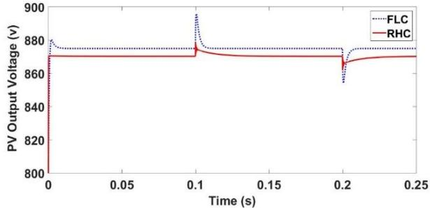
Fig. 8 Comparison of PV output voltage for the two controllers by considering uncertainties (change in irradiation).
