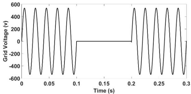
Fig. 12 Grid voltage in phase a,  $E_a$ , for the RHC during three-phase short-circuit fault.
