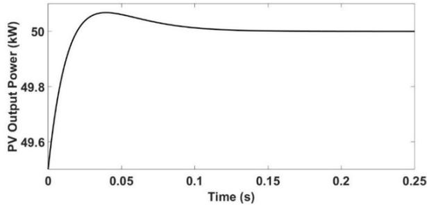
Fig. 7 PV output power for the RHC in standard atmospheric conditions.
