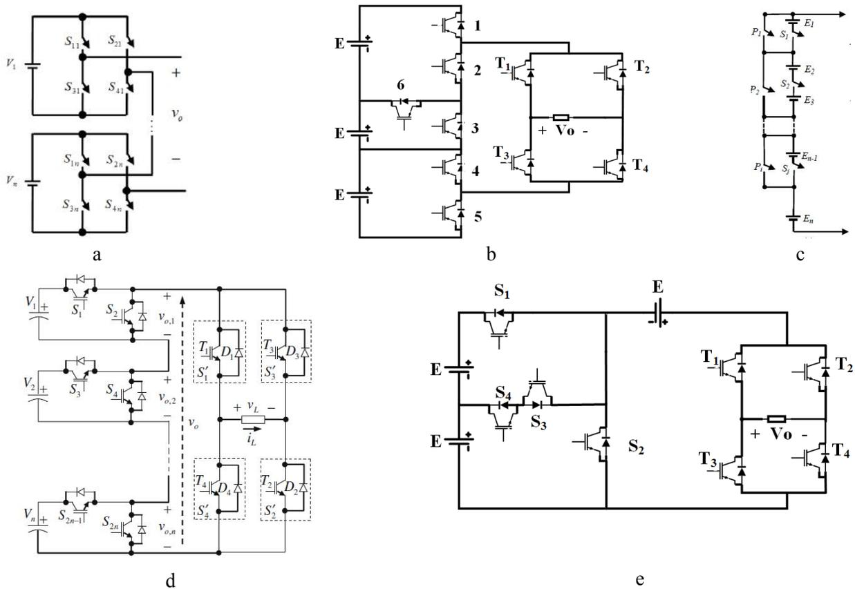
Fig. 4: Symmetrical cascaded multilevel inverters; a) proposed inverter in [29] - (R<sub>1</sub>- CHB); b) proposed topology in [30] - (R<sub>2</sub>); c) presented topology in [31] - (R<sub>3</sub>); d) suggested structure in [32] - (R<sub>4</sub>); e) proposed topology in [10]- (R<sub>5</sub>)
