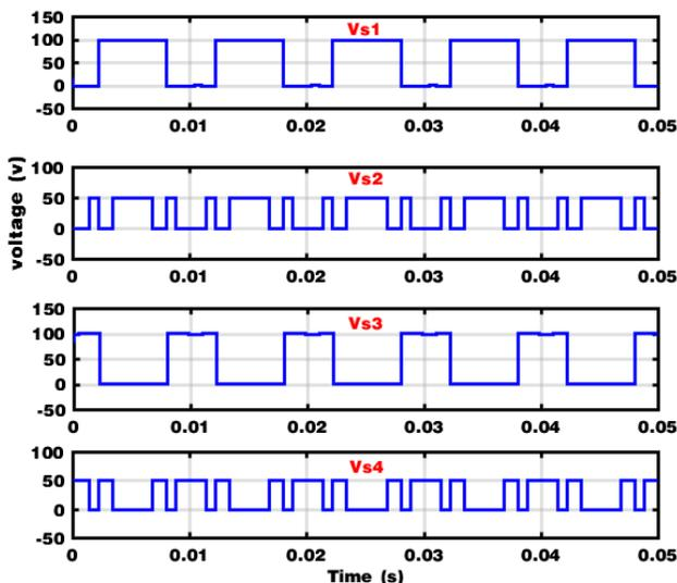
Fig. 12: Voltage across level generator switches.
