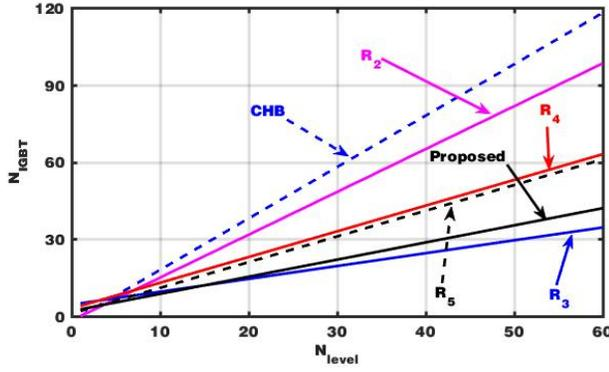
Fig. 6: Comparison of  $N_{IGBT}$  in different topologies
