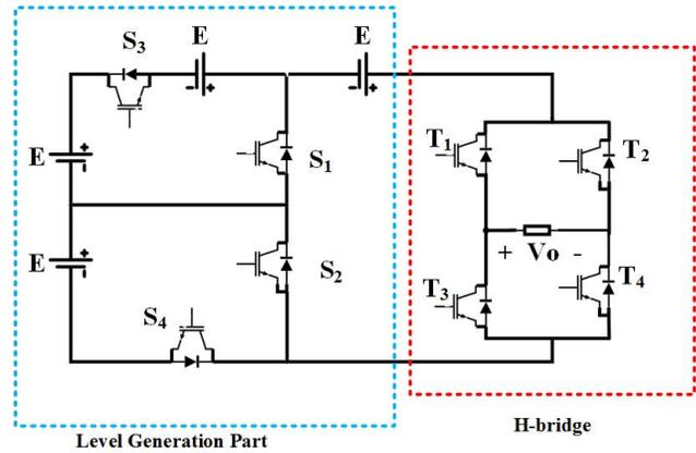
Fig. 1: Basic unit of the proposed topology
