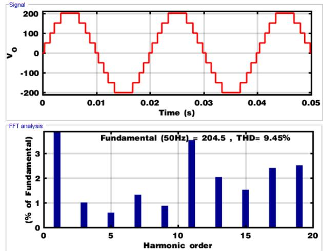
Fig. 9: Simulation output voltage waveform with harmonic spectrum
