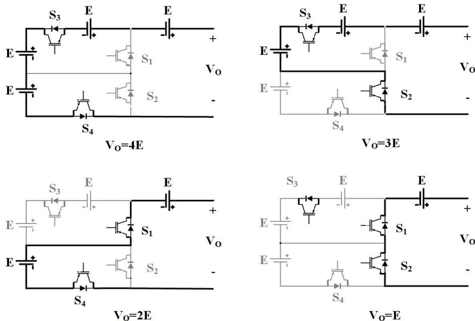
Fig. 2: Different operating modes of proposed inverter
