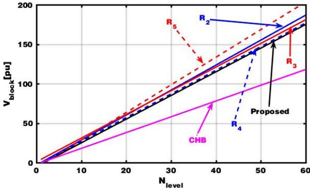
Fig. 7: Comparison of  $V_{block}$  in different topologies
