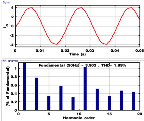
Fig. 10: Simulation output current waveform with harmonic spectrum
