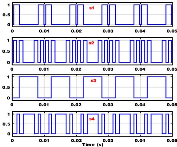
Fig. 11: Gate signals of level generator switches
