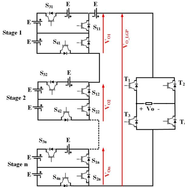
Fig. 3: The proposed cascaded inverter
