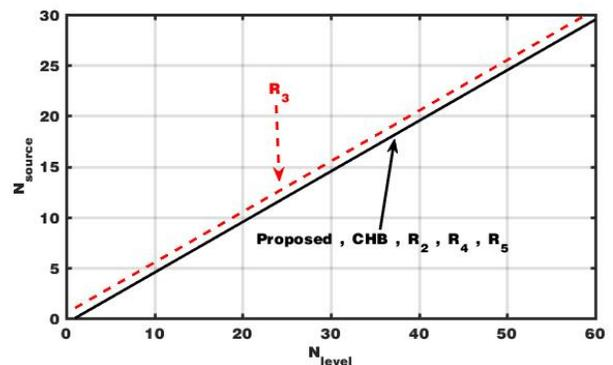
Fig. 5: Comparison of N<sub>source</sub> in different topologies
