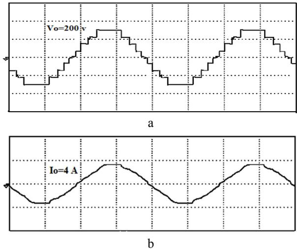
Fig. 14: Experimental results of proposed 9-level topology; a) Output voltage waveform; b) Output current waveform
