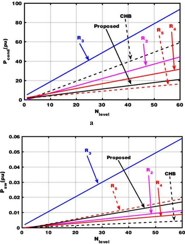
Fig. 8: Comparison of the losses in different topologies; a) The conduction losses; b) The switching losses
