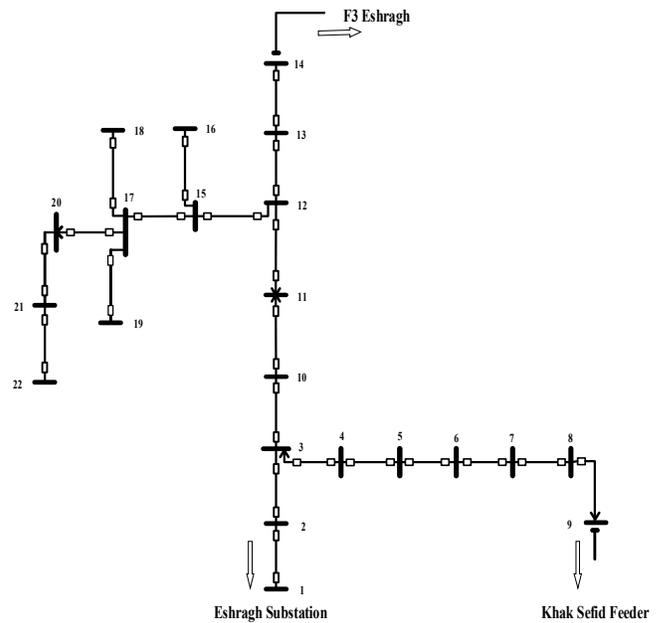
Fig 5. The single-line diagram of a real feeder 4 of ESHRAGH sub-transmission substation in the GTEDC
