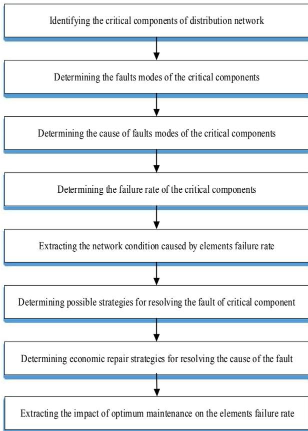
Fig1. The flowchart of the basic analysis of the proposed RCM algorithm.
