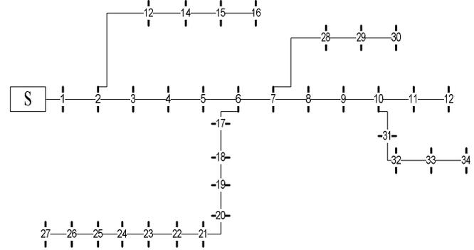
Fig. 7. Single-line diagram of a 33-bus Standard network
