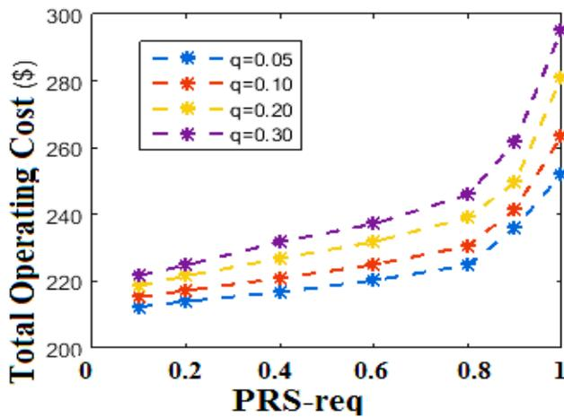
Fig 10: Comparison of total operating cost with different PRS<sup>req</sup> and different q values
