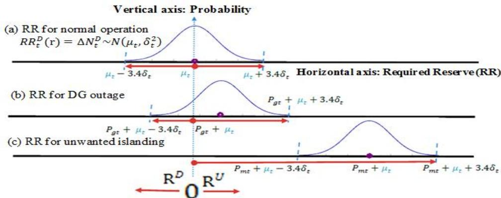
Fig 1: PDFs of required reserve for normal operation, DG outage, and unwanted islanding
