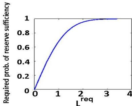
Fig2: The relation between  $L^{req}$  and the required probability of the reserve sufficiency ( $PRS^{req}$ )
