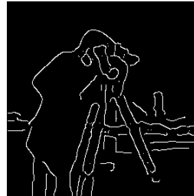
Extracted edges using canny method
